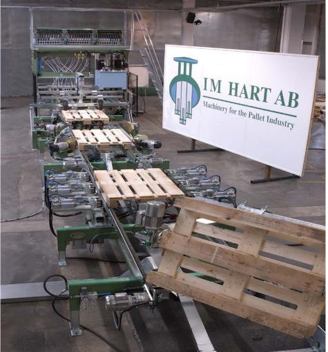
This eminent and complete after treatment line from IM Hart AB contains: Chamfering-, corner-cutting-, branding-, turner-, stacker- and chain conveyor machine. It stands for flexibility strength, and the high capacity, along with a top quality production, despite producing EUR-pallets or one way pallets.
